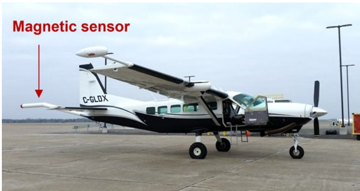
A typical survey airplane. Similar planes have been flying around Far West Texas to map critical rare earth minerals. The magnetic sensor is placed in an extension on the back of the airplane to reduce the impact of the airplane's own magnetic field.
